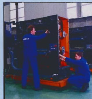
Installation of printing units on an eight-page press of the 6611 series.
