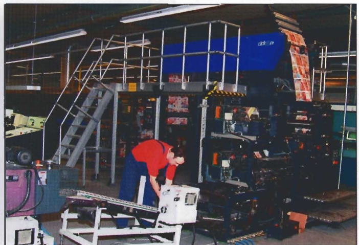
Shortly before the press was to be put into operation, some more adjustments were made on the folder with its two deliveries.
